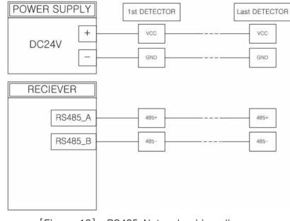
[Figure 13] RS485 Network wiring diagram
