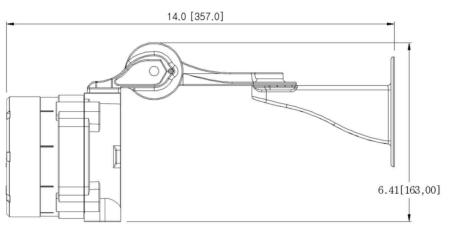
[Figure 4] Combination of Detector with Bracket, inch[mm]
