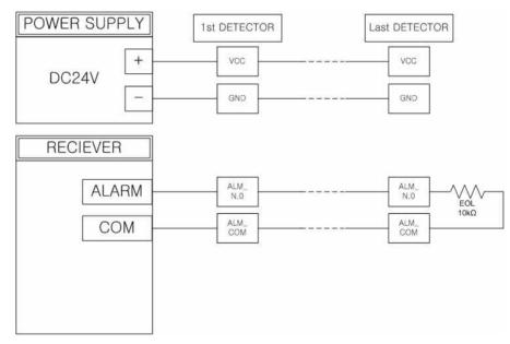
[Figure 9] Wiring diagram for fire detection only
