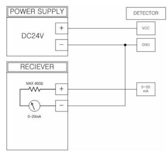
[Figure 12] Current output wiring diagram
