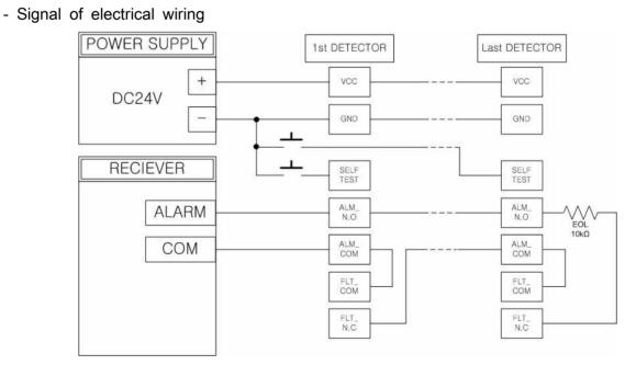
[Figure 15] External self test wiring diagram
