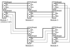
The diagram shows an example of the wiring for a closed VESDAnet loop, which is the recommended configuration. Remove the factory default A and B links from the VESDAnet sockets (C and D) prior to connecting the detector to the VESDAnet. It is recommended that 120 Ohm twisted pair cables (e.g. Belden 9841) be used for including the devices in the network, with a maximum length between devices of 1.2 km The polarity of the data wires must be maintained throughout the network.
