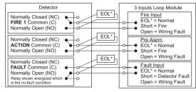
This wiring example is for wiring VESDA detectors to a typical third party Input Loop Module with three
