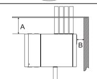
Ensure that there is sufficient clearance to mount the detector, noting the location of air sampling pipes and cable entry points. Due to the rigid nature of the plastic pipe, installation must provide for sufficient movement in all pipework (air inlet, air exhaust and cable pipes) to allow pipe ends to be easily fitted and removed.
