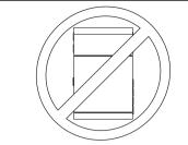
The VESDA-E detector can be mounted in an upright or inverted position. Do not mount the detector with a sideways orientation.
