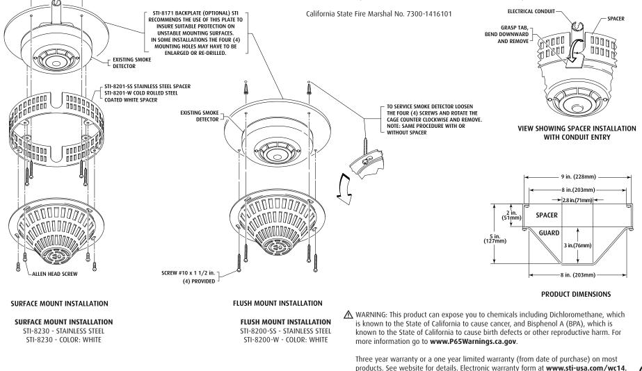
**INSTALLATION OF STI-8200 SMOKE DETECTOR GUARD**
