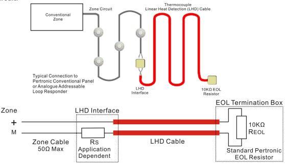
The following Table can be used to select the Series Resistor (Rs) value:
