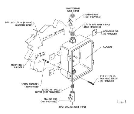
3. Pull 24 VDC and alarm wiring into back box through top conduit; and pull 110 or 240 VAC wiring into back box through bottom conduit per NFPA 70, NEC and local codes.
