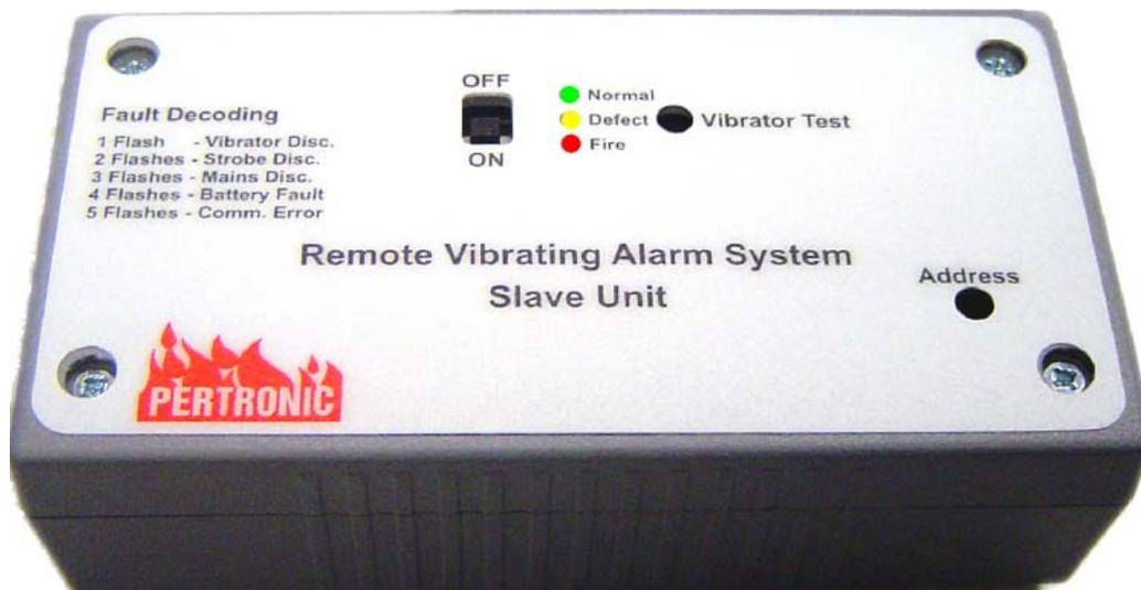
Figure 3.2: Front Panel Layout of Slave Unit
