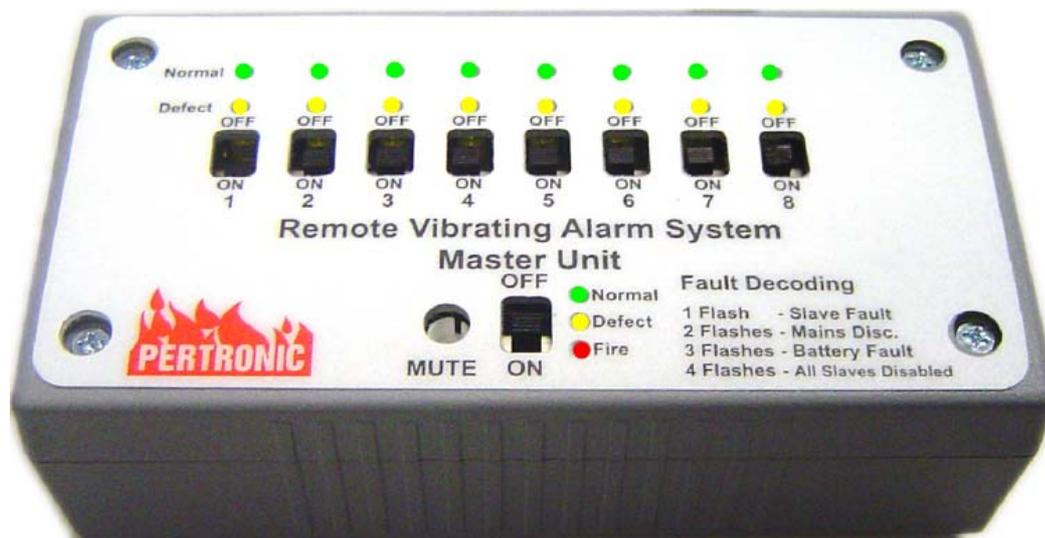
Figure 2.2: Front Panel Layout of Master Unit
