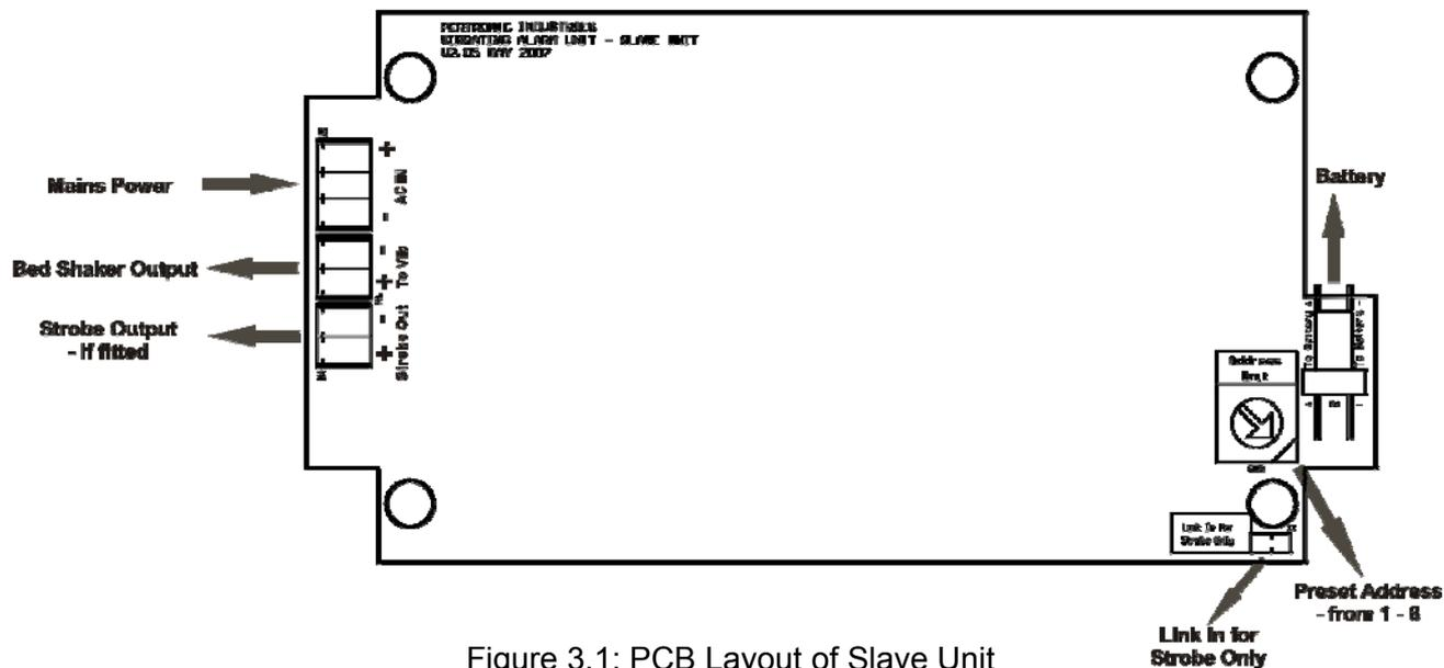
Figure 3.1: PCB Layout of Slave Unit
