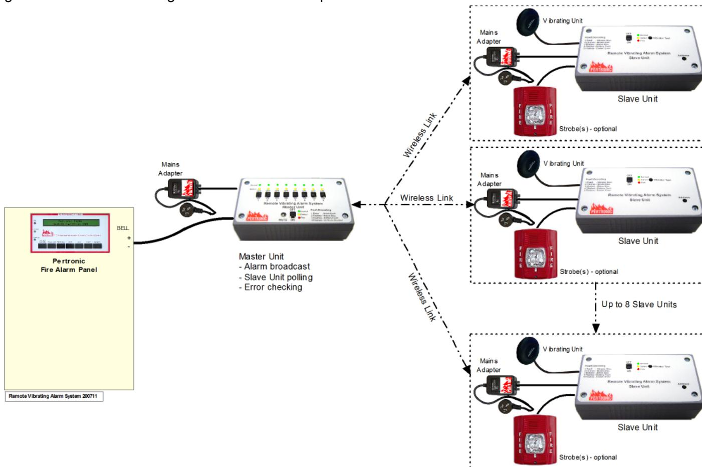
Figure 5.1: Typical Panel Connection
