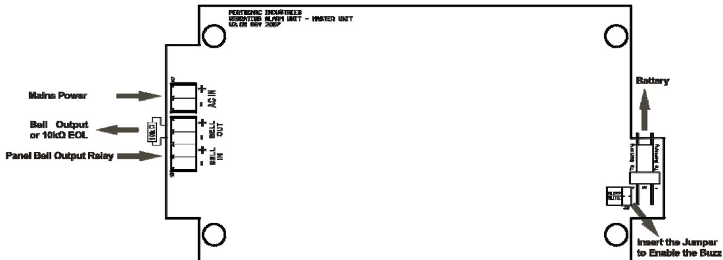
Figure 2.1: PCB Layout of Master Unit (Rear)
