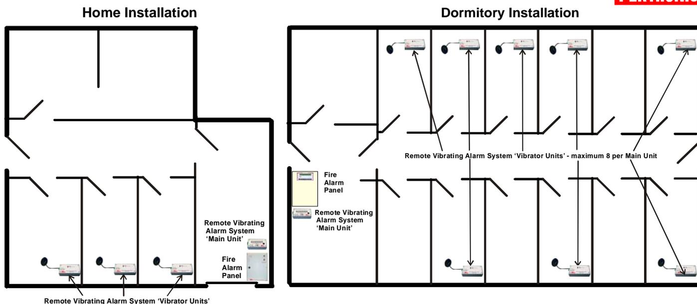
Figure 5.2: Sample Installation Layouts
