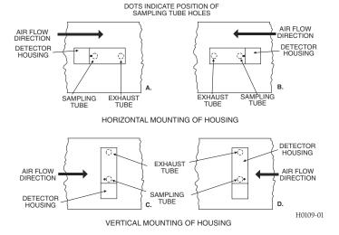
NOTE: Only metal sampling tubes may be used on orientations C and D.
