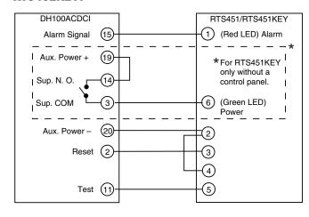
Figure 10. Multiple fan shutdown (interconnect):
