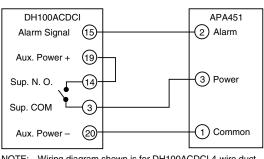
NOTE: Wiring diagram shown is for DH100ACDCI 4-wire duct smoke detector system equipped without a control panel.
