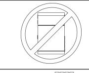
The VESDA-E detector can be mounted in an upright or inverted position. Do not mount the detector with a sideways orientation.
