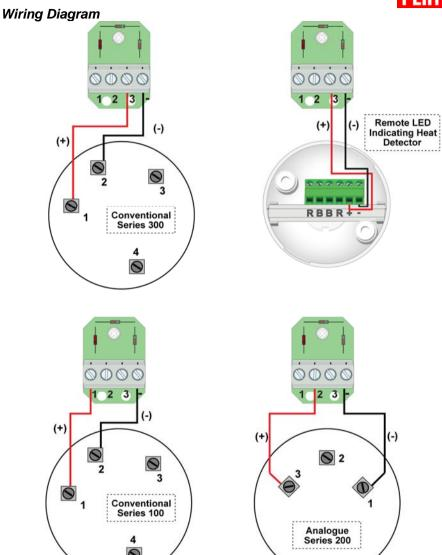
NOTE: The wiring shown is additional to the normal detector field wiring. Refer to the corresponding Detector Installation Notes for connection diagrams.
