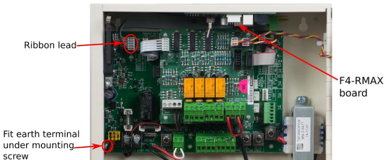
Figure 4: F4 panel with RMAX and Type 5 boards.
