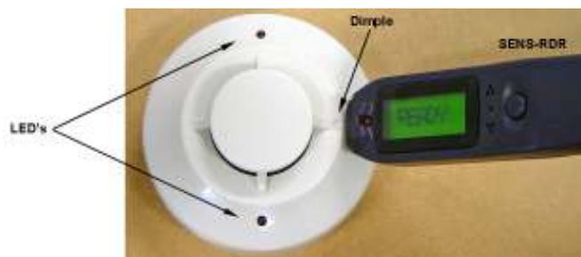
We all know that many false alarms are generated by dirty or dusty conventional detectors. With this new detector model, the Sensitivity Reader will quickly help the service technician identify, in the future, which detectors are dirty and prone to false alarming, to allow preventative detector maintenance.
