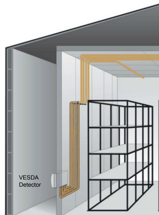
Figure 3. VESDA detector located externally to the protected area
