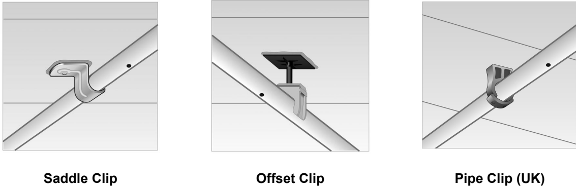
Figure 4: Pipe Network Supports
