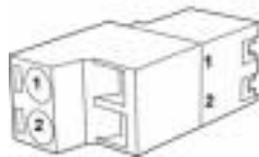
Figure 7 - Terminal and plug set up, GPI connections
