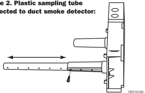
**[5.3] Secure The Detector Housing To The Duct**
