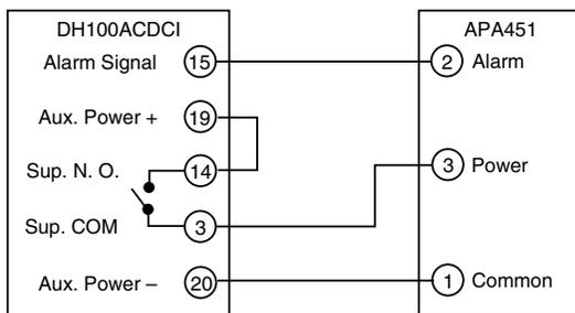
NOTE: Wiring diagram shown is for DH100ACDCI 4-wire duct smoke detector system equipped without a control panel.
