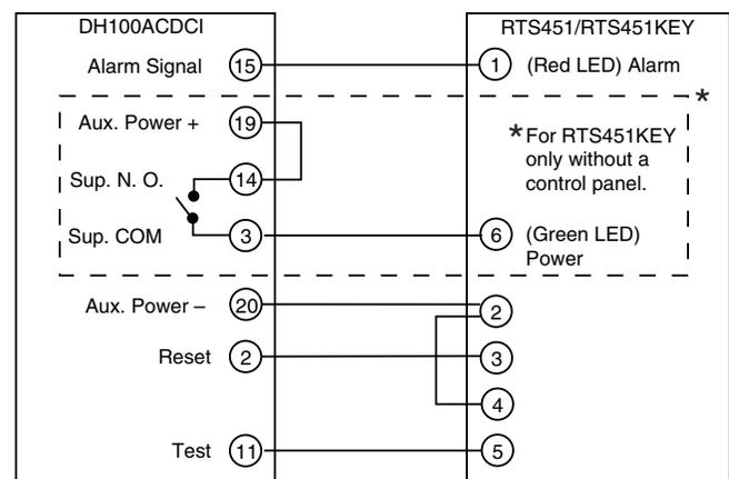
**Figure 10. Multiple fan shutdown (interconnect):**
